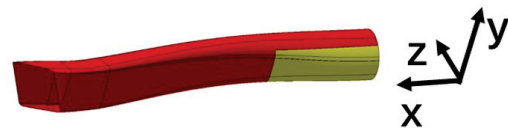
Fig. 13. Partial coating scheme for cavity in Fig. 12 (red area is coated).
