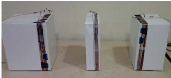
Fig. 6. Experimental setup for multiple coils [39].
