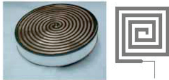
Fig. 5. Example of a microstrip circular spiral coil antenna and square spiral antenna [38].
