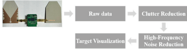
Fig. 11. Block diagram of UWB radar signal processing.
