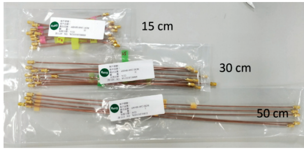
Fig. 2. Coaxial cables used for measurement.
