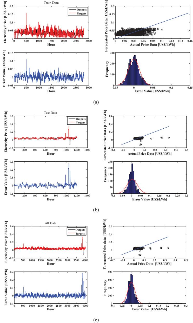
**Figure 9** Forecasting results of electricity price using RBF neural networks: (a) training data; (b) testing data; (c) all data.
