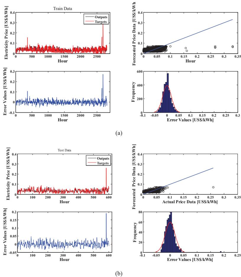
**Figure 8** Forecasting results of electricity price using MLP neural networks: (a) training data; (b) testing data; (c) validation data; (d) all data.
