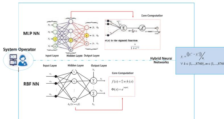
Figure 6 The proposed hybrid framework based on MLP-RBF neural networks.
