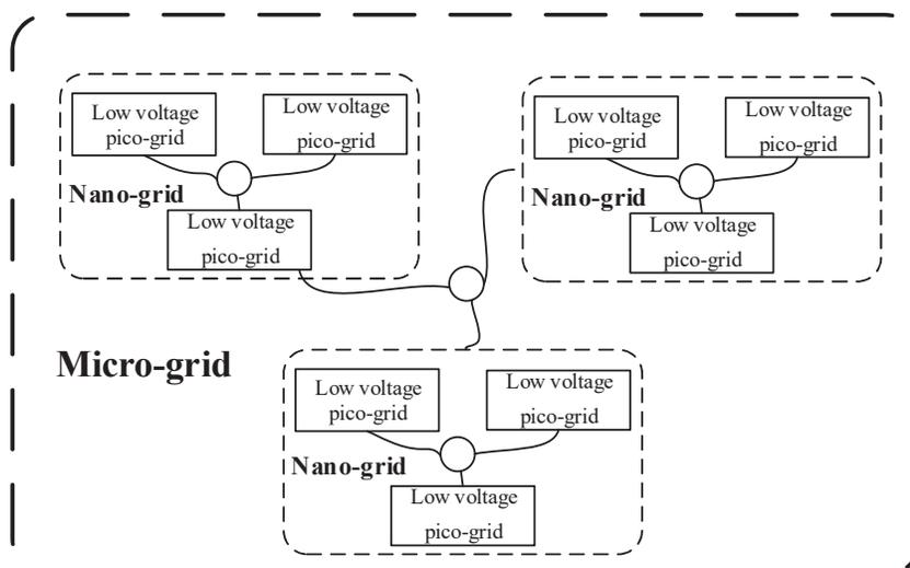
**Figure 1** Example of multiple pico-grids forming a micro-grid.
