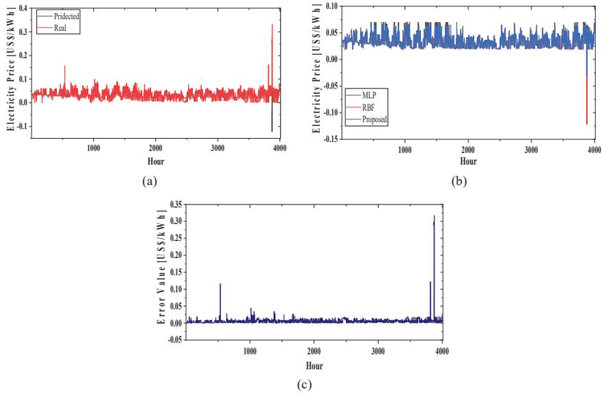
Figure 11 (a) Forecasting results of the hybrid model and real electricity price data; (b) Comparison of the proposed model with MLP and RBF models; (c) Error values of the predicted values.
