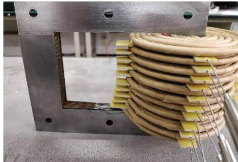
Figure 5 The photo of winding thermocouple installation.
