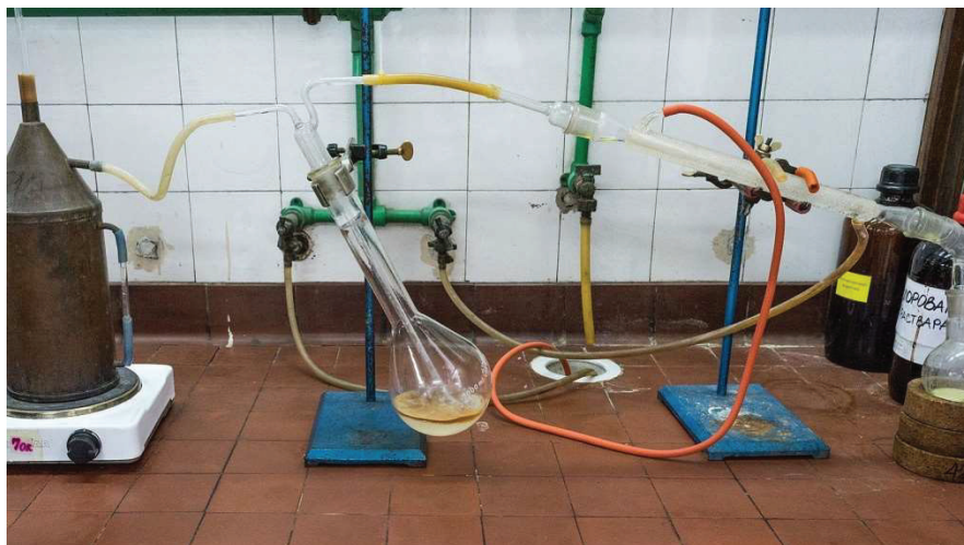
Figure 2 Separation of bio-ethanol by vacuum distillation.
