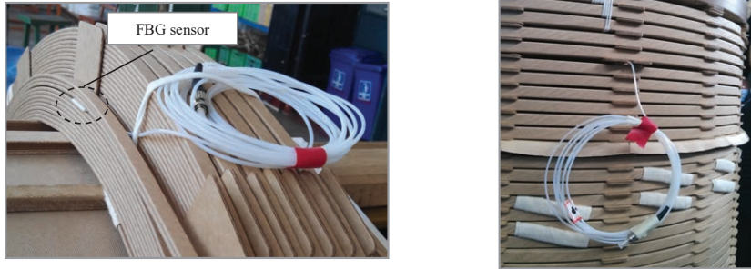
(a) The clamping of the sensor in the winding (b) Sensor tail optical fiber
