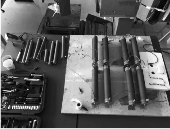
Figure 14. Resistor module with known resisting value
