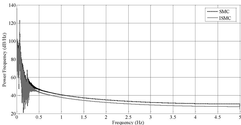
Figure 11. Power spectral density of generator torque for SMC and ISMC using FAST.
