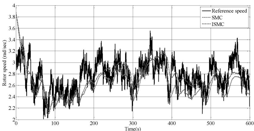
Figure 10. Rotor speed comparison for SMC and ISMC using FAST simulator
