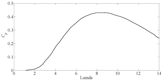
**Figure 2.  $C_p$  vs  $\lambda$  curve**
