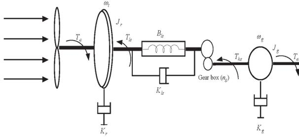
Figure 3. Two mass model of the WT.
