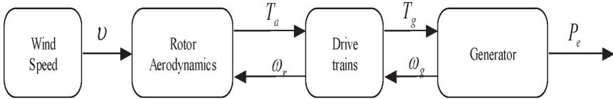
**Figure 1. Schematic of WT.**
