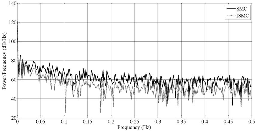
Figure 9. Power spectral density of generator torque.
