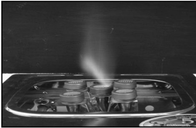
Figure 8. Vertical Burner Flame, 0.2 bar, 1.0mm Nozzle, Low Setting.
