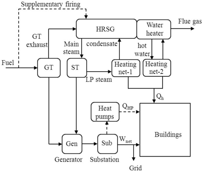
Figure 1. Schematic diagram of distributed energy system
