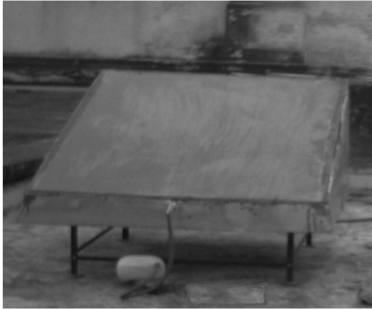
Figure 1b. Photograph of passive solar still.
