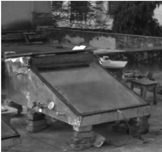
Figure 2b. Photograph of new design solar still.
