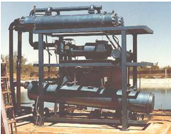
Figure 3. The solar pond built at Alice Springs in central Australia (left) in the 1970's and (right) the Organic Rankine engine used to generate power from the pond's hot water.
