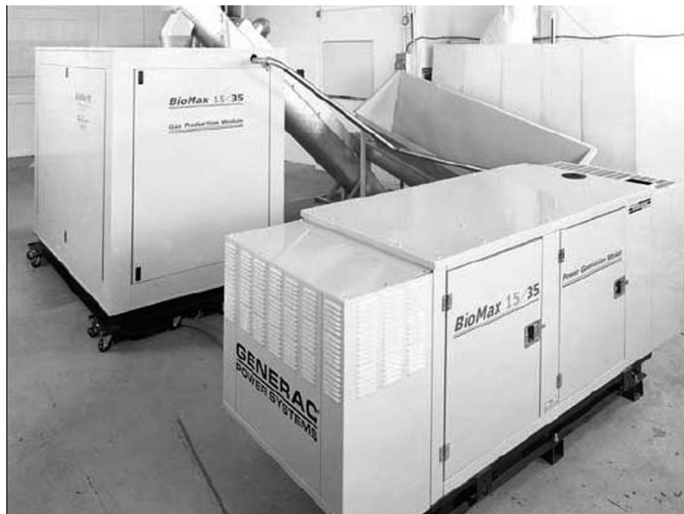
Figure 15. A 15-kW Generator and Gasifier
