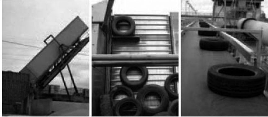
Figure 8. TDF Feeding System
