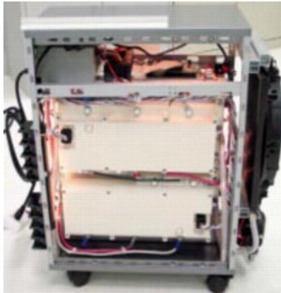
Figure 9. 200 kW Induction Generator Controller
