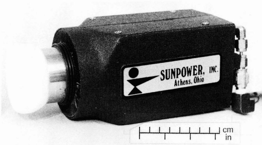
Figure 7. Electrically driven free-piston Stirling cooler. Heat is accepted at one end (note the ball of ice that has formed), and rejected with the aid of a fan from the other. The integral linear motor drives the piston and implements the Stirling cycle. Like a free-piston Stirling engine, the piston and displacer float on gas bearings, are resonated with planar springs, and are hermetically sealed with the linear motor. Helium serves as the working gas and for operation of the gas bearings.
