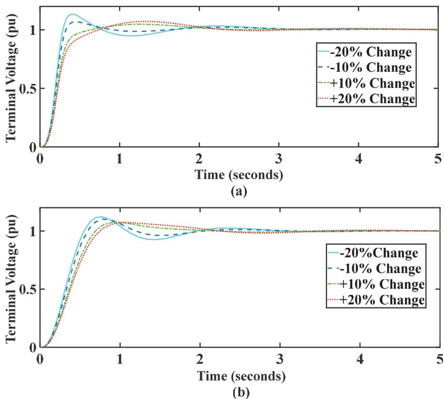
**Figure 6** Transient response plots obtained after varying exciter time constant values of; (a) SF-SMC controlled system, (b) LQR controlled system.
