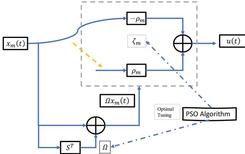
**Figure 2** Block diagram illustrating proposed PSO based SMC methodology.
