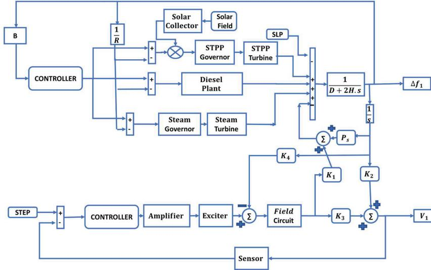
Figure 1 Block diagram of combined AVR-LFC model.
