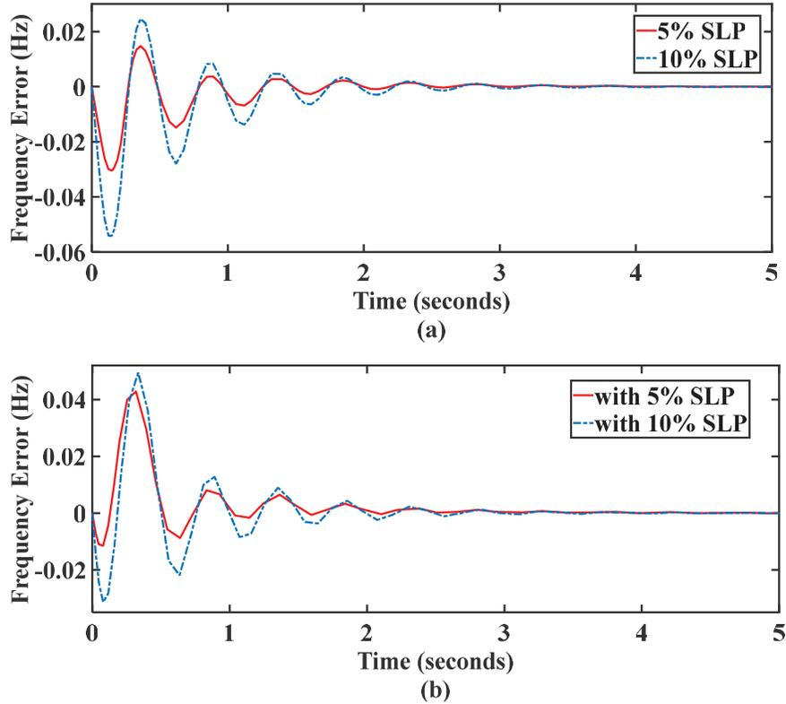
**Figure 5** Transient response plots of frequency error obtained after varying the SLP value of LFC loop using; (a) SF-PID, (b) LQR.
