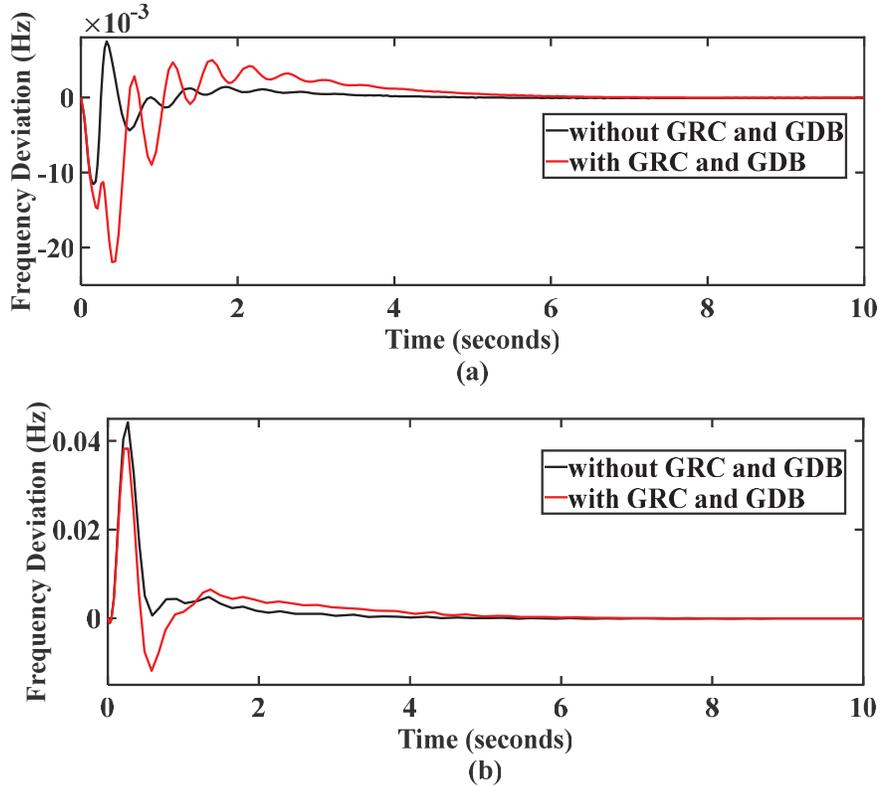
**Figure 7** Transient response plots obtained after considering nonlinearities in; (a) SF-SMC controlled system, (b) LQR controlled system.
