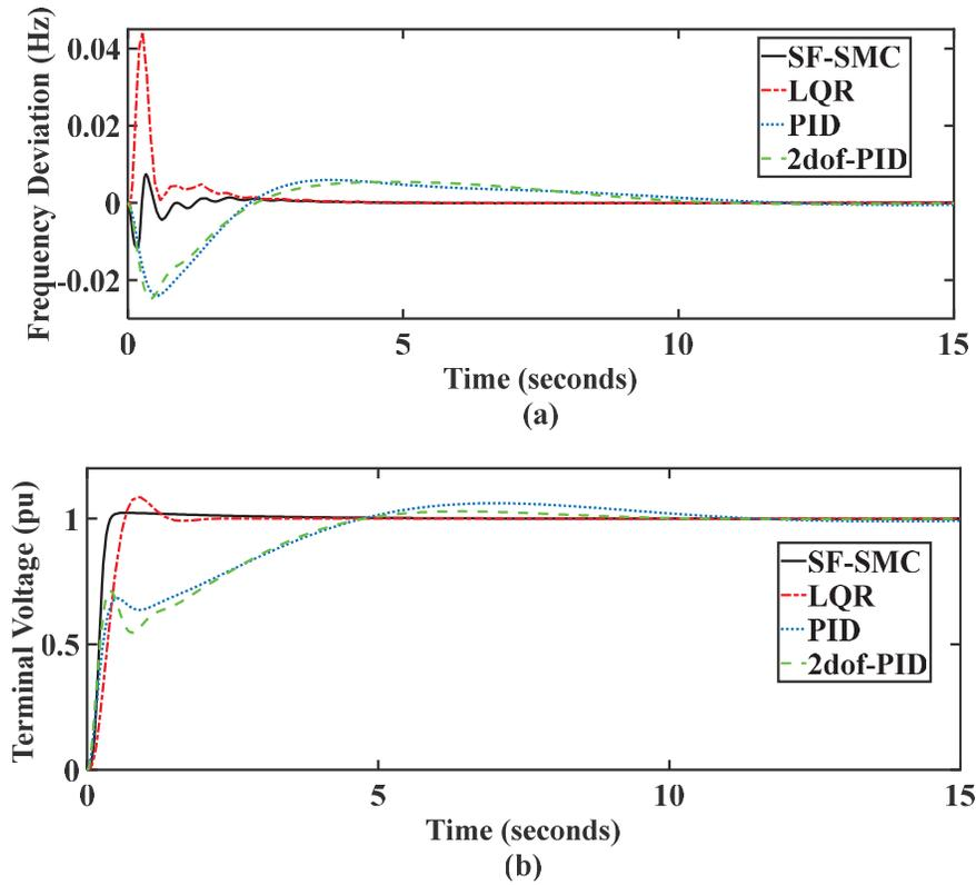
**Figure 4** Transient response plots obtained after using LQR, SF-SMC, PID, and 2-DOF PID controllers for; (a) frequency deviation, (b) terminal voltage.
