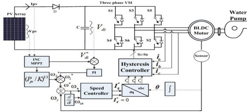
Figure 1 Structure for PV based water pumping system.
