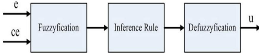
**Figure 3** Structure of fuzzy logic control.
