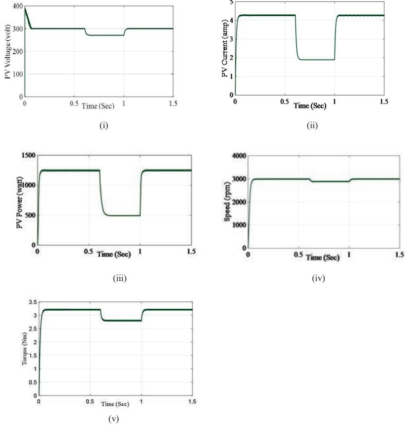
**Figure 6** Responses of (i) PV voltage (ii) PV current (iii) PV power (iv) Motor speed (v) Motor torque, for  $1000 \text{ W/m}^2$  insolation under dynamic-state.
