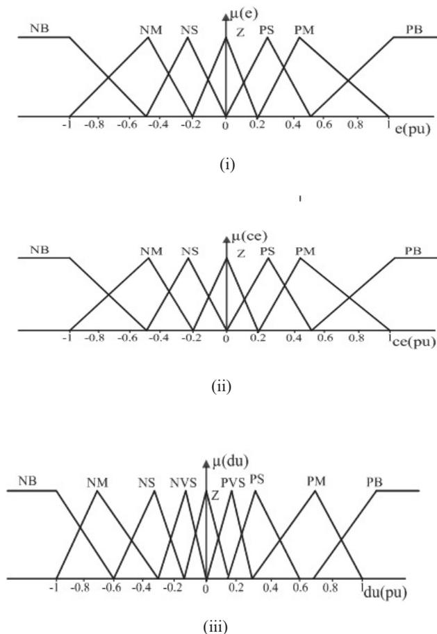
**Figure 4** Membership Function of (i)  $e$ , (ii)  $ce$ , and (iii) output.
