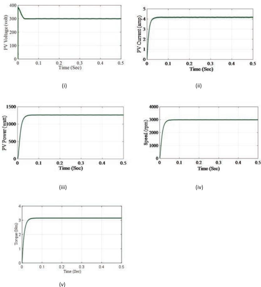
**Figure 5** Responses of (i) PV voltage (ii) PV current (iii) PV power (iv) Motor speed (v) Motor torque, for  $1000 \text{ W/m}^2$  insolation under steady-state.
