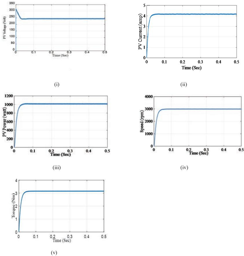
**Figure 7** Responses of (i) PV voltage (ii) PV current (iii) PV power (iv) Motor speed (v) Motor torque, for  $1000 \text{ W/m}^2$  insolation under partial shading condition.
