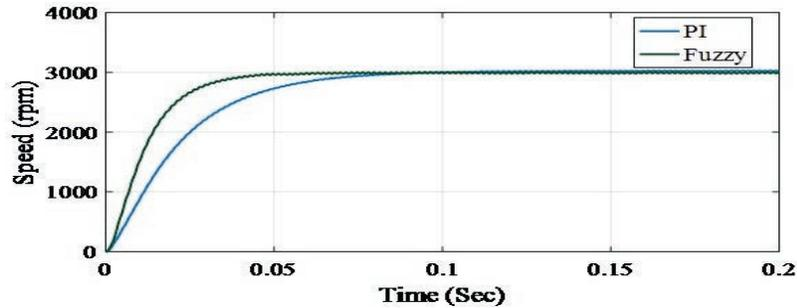
**Figure 8** Speed response of PI and Fuzzy logic controller.
