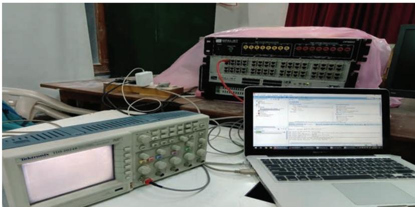
**Figure 9** OPAL-RT interfaced with console PC.
