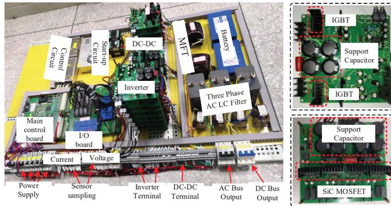
**Figure 7** Prototype photograph of the DAB system.
