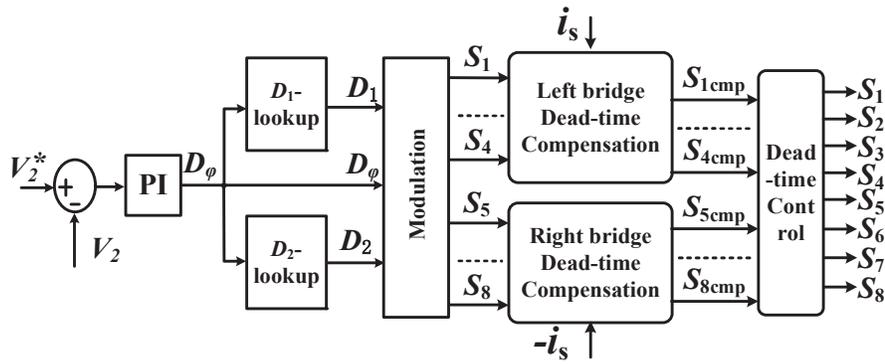
Figure 4 Control block diagram of DC-DC converter.
