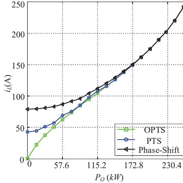
**Figure 6** Comparison curve of leakage inductor current RMS under OPTS, TPS and phase-shift control.
