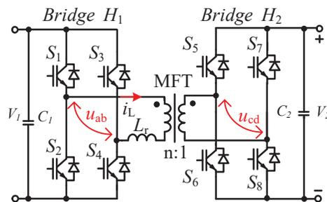
Figure 1 Topology of bidirectional isolated DAB converter.
