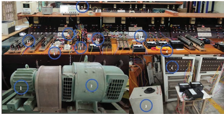
Figure 10 Experimental setup of the proposed system. 1-DC motor, 2-Induction Generator, 3-three phase auto transformer, 4-Fluke 345 clamp meter, 5-Capacitor bank, 6-consumer load, 7-Digital storage oscilloscope, 8-three phase diode bridge rectifier, 9-multi meter, 10-High voltage differential probe, 11-Hall effect current probe, 12-DC loads.
