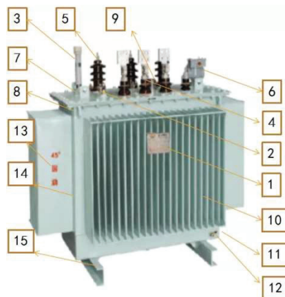
1 – Tabelet; 2 – Thermometer base; 3 – Tubular oil level gauge; 4 – Low voltage bushing; 5 – HIGH voltage bushing; 6 – Gas relay; 7 – Hoisting and mixing of the body; 8 – Transformer hoisting and mixing; 9 – Tap changer; 10 – Oil tank; 11 – Oil drain valve; 12 – Grounding identification; 13 – Transformer oil number; 14 – Body; 15 – Footing.
