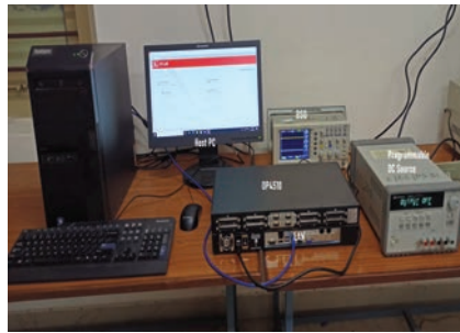
(a) OPAL-RT real-time experimental setup
