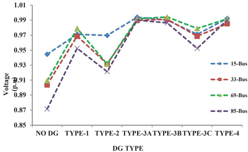
Figure 7  $V_{min}$  for all bus systems with all types of DGs and without DG.
