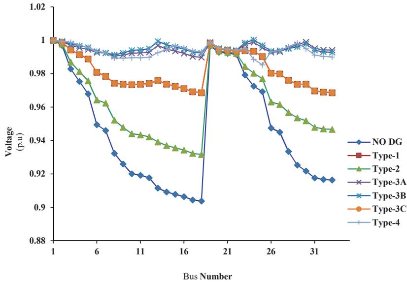
Figure 2 Voltage profile for 33-Bus system.
