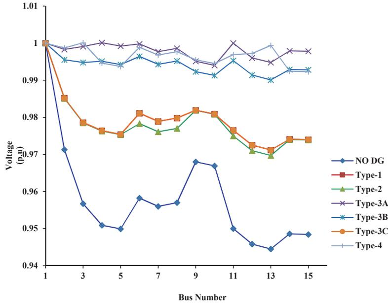
Figure 1 Voltage profile for 15-Bus system.
