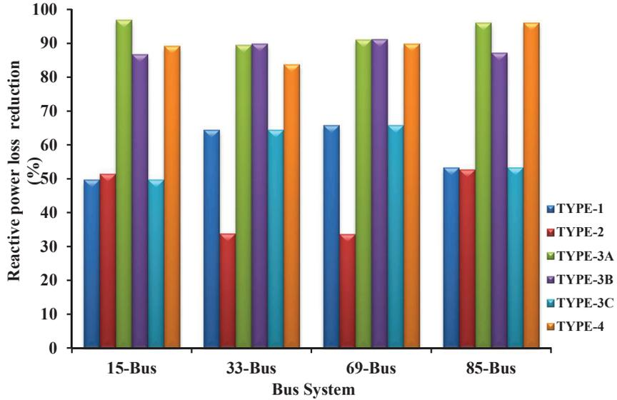
Figure 6 Reactive power loss reduction (%) of all bus systems.
