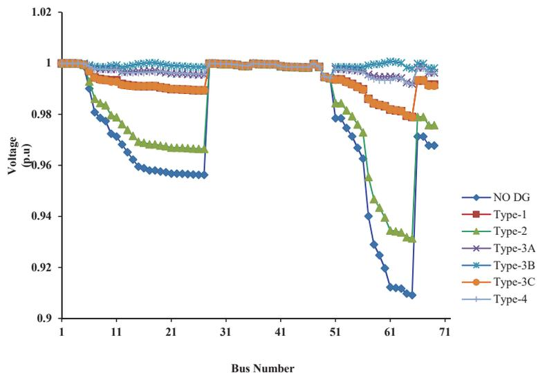
Figure 3 Voltage profile for 69-Bus system.
