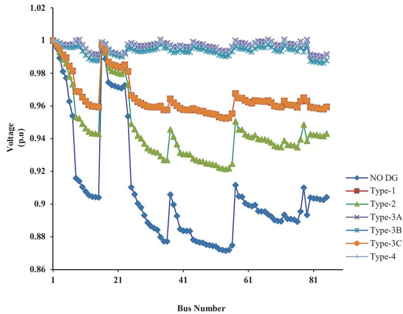
**Figure 4** Voltage profile for 85-Bus system.
