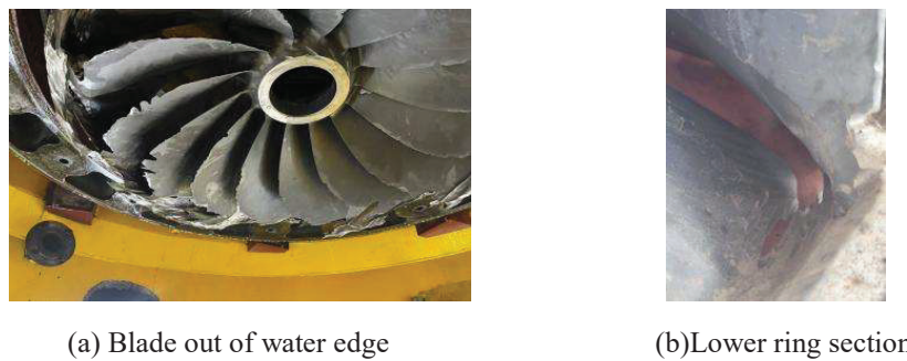
Figure 12 Wear of crown and ring gap on actual turbine blades.
