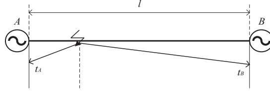
Figure 3 Schematic diagram of double-ended traveling wave localization.
