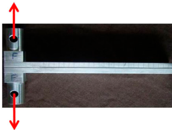
Figure 6. DCB adhesive joint tested (Shyanbhog, 1998).
