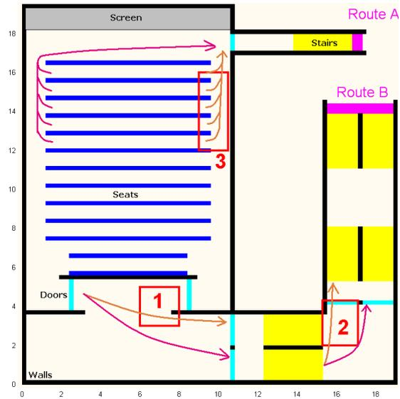
**Figure 4.** Snapshots of numerical simulations; seats, walls, screen, stairs, and doors are represented; escape routes are the route A at the top and route B bottom; depending on the number of students in the rectangles (number 1, 2 or 3), students move in the direction of the dark-colored arrow instead of the light-colored one
