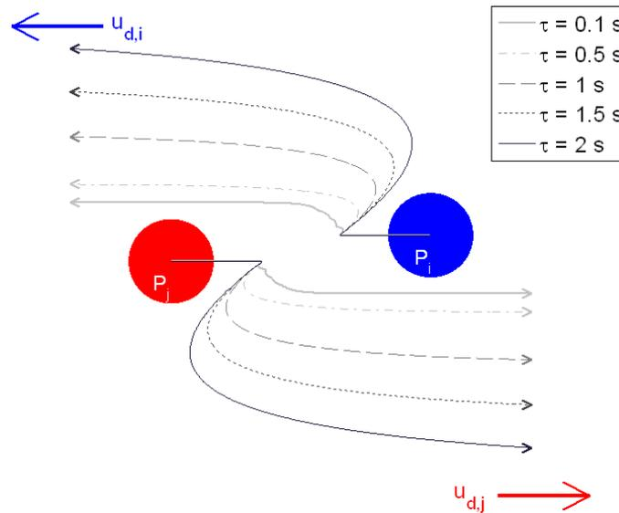
**Figure 1.** Representation of the trajectories of two identical pedestrians  $i$  and  $j$  moving in opposite directions with different values of  $\tau$ . After collision, for each pedestrian, the external acceleration force allows the pedestrian to gradually switch from the actual velocity after shock to the desired velocity, depending on the values of  $\tau_i$  and  $\tau_j$ . In this example,  $\tau_i = \tau_j = \tau$
