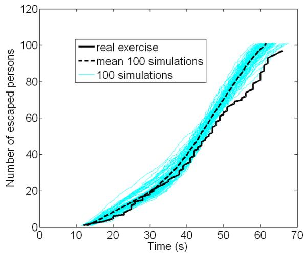
**Figure 6.** Number of persons out vs. time (egress curves), comparison between real exercise result and numerical simulations results: the 100 numerical simulations are the light-colored curves, the mean of these simulations curves is the black bold dotted curve, and the real exercise curve is the black bold one
