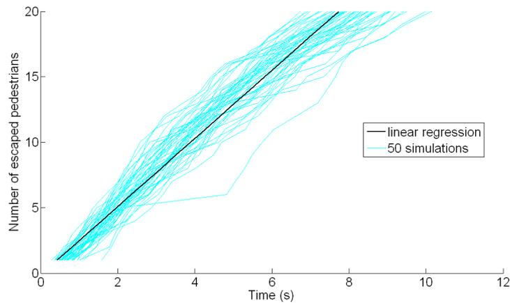
**Figure 3.** Simulated evacuation time for a room with a door of 82 cm width. Shown is the total number of pedestrians out vs. time for the adapted NSM2. The 50 simulations are the light-colored curves. The linear regression of the 50 simulations (black line) allows us to obtain the average flow through the door**Table 5.** Average flow (pedestrian/s) through a door of 82 cm
