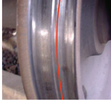
Figure 3 Abnormal wear of wheel-rail tread.
