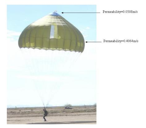
Figure 3. TP8 flight test
