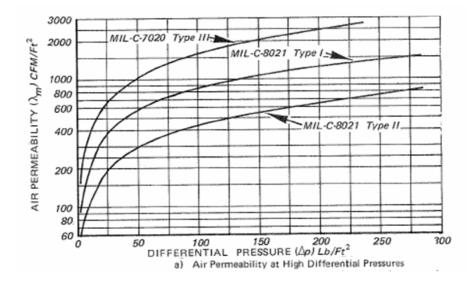
Figure 1. Parachute fabric permeability data (AFFDL-TR-78-151 report, 1978)
