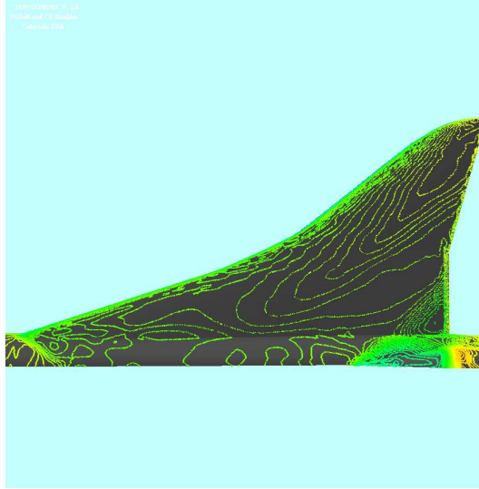
Figure 7. Flow around Dassault SSBJ geometry, Mach 1.6, incidence 0: Mach number contours on upper side obtained by applying the previous version of the scheme
