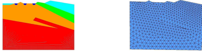
Figure 9. Foothills areas. Left, 2D uniformly refined mesh showing the velocity contrast between the layers, the velocity in near surface is lower than in the substratum; Right, 2D initial coarse mesh for the adaptive computing
