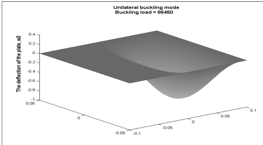
**Figure 8.** The unilateral buckling mode of the plate in the case:  $\omega_c = \bar{\omega}$
