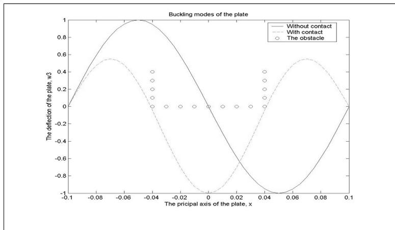
**Figure 5.** The sections A of the buckling modes of the plate in the case:  $\omega_c = \omega_{c1}$
