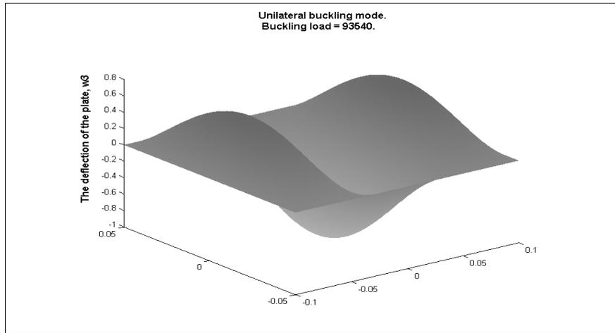
**Figure 4.** The unilateral buckling mode of the plate in the case:  $\omega_c = \omega_{c1}$
