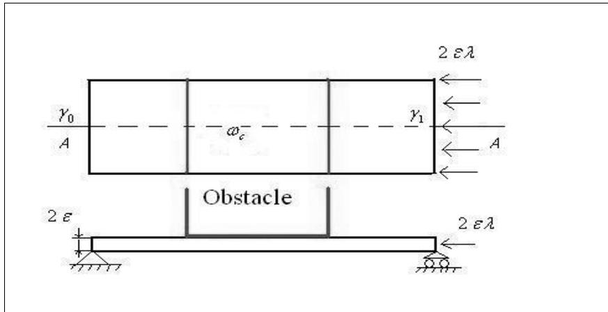
**Figure 2.** The rectangular plate is in presence of the obstacle
