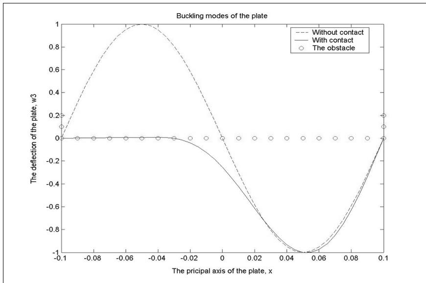
**Figure 9.** The sections A of the buckling modes of the plate in the case:  $\omega_c = \bar{\omega}$
