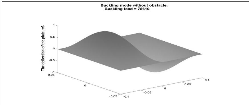
**Figure 3.** The buckling mode of the plate in the absence of any obstacle
