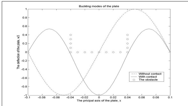
**Figure 7.** The sections A of the buckling modes of the plate in the case:  $\omega_c = \omega_{c_2}$
