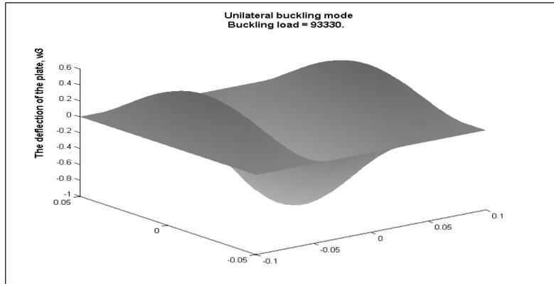
**Figure 6.** The unilateral buckling mode of the plate in the case:  $\omega_c = \omega_{c_2}$
