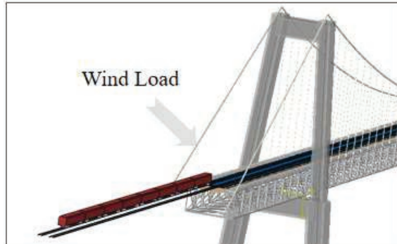
Figure 5 Wind-vehicle-bridge coupling model based on secondary development.
