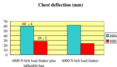
**Figure 12.** Effect of various restraint systems on the thoracic deflection
