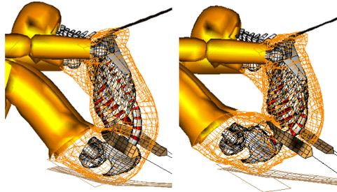
**Figure 8.** *Illustration of submarining phenomenon*
