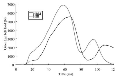
**Figure 10.** Comparison of outer lap belt loads
