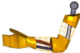
**Figure 6.** Deformable arm model
