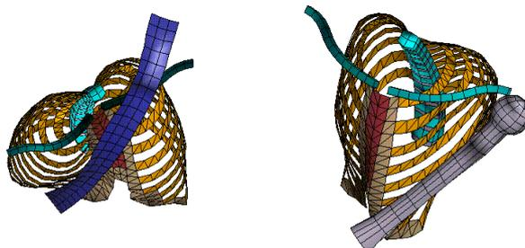
**Figure 7.** Rib cage loaded by a seatbelt (on the left) and a door in side impact (on the right)
