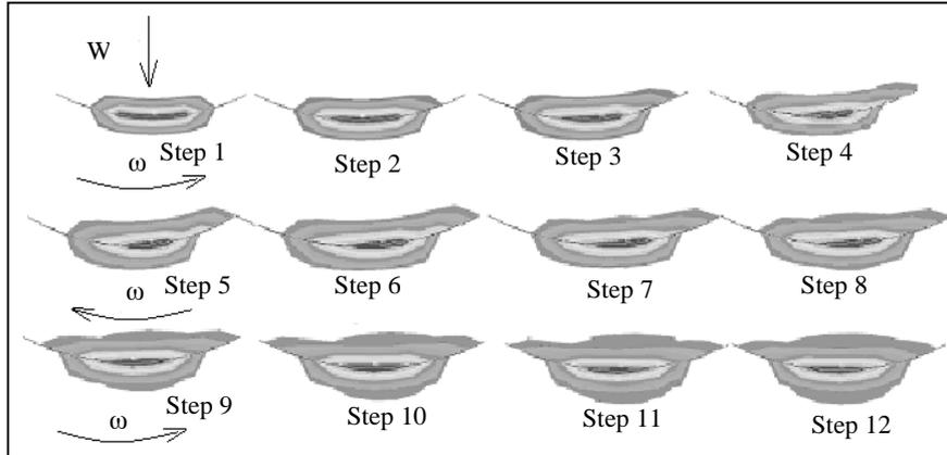
Figure 6. Temperature contour during 1 cycle of rotation
