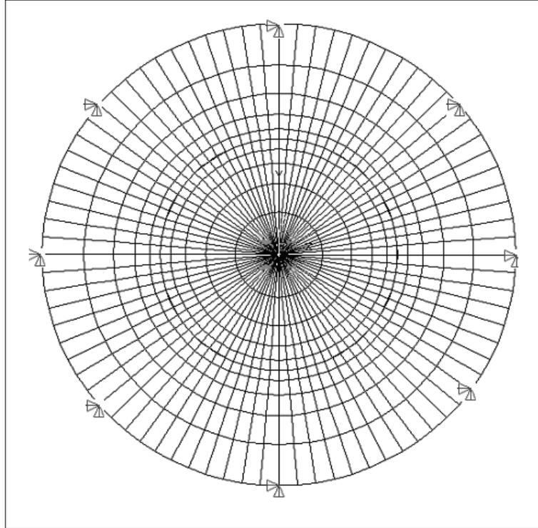
**Figure 5.** *Mesh pattern for the oscillating pin-bushing assembly*
