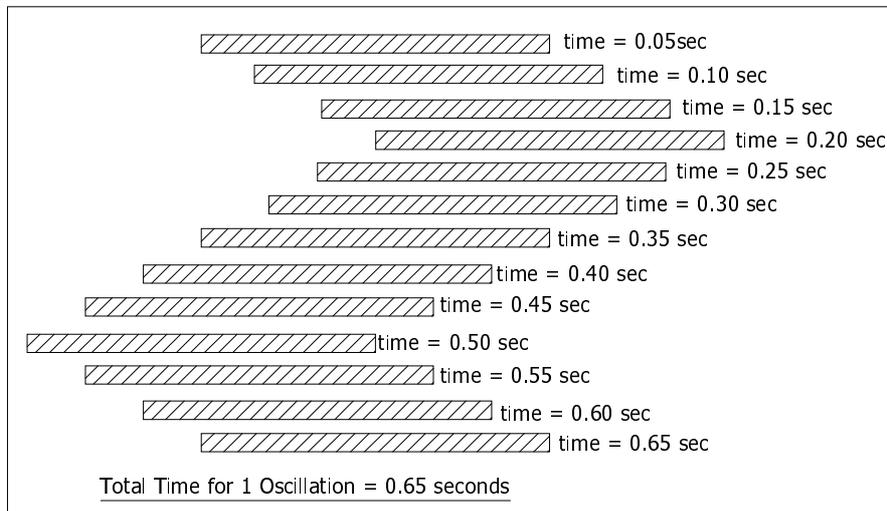
**Figure 3.** Application of oscillating heat flux as a function of time and space. In this illustrations, the number of time steps for 1 complete oscillation,  $i$ , is 13
