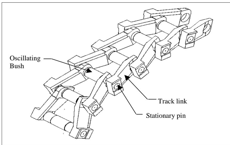
**Figure 1.** Track retention assembly with oscillating pin and bushing
