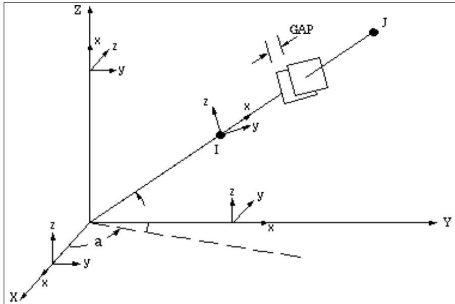
**Figure 4.** Schematic of 2-noded contact element connecting nodes "I" and "J"
