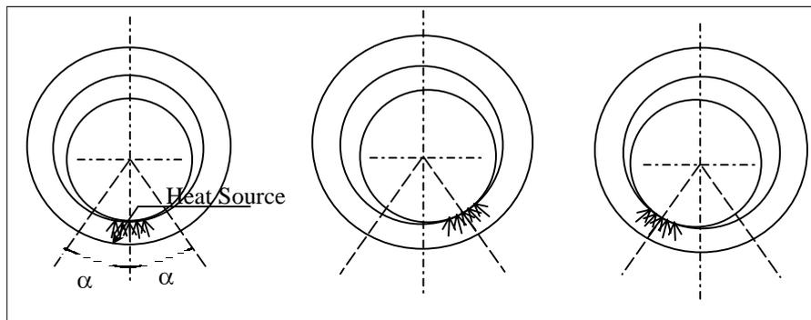
**Figure 2.** Schematic of application of oscillating flux,  $\alpha$  is the oscillation angle
