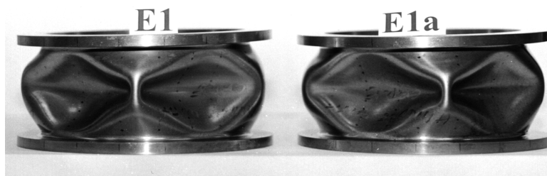
Figure 14. View of two, nominally identical mild steel barrels, after the collapse (from Blachut 2003, p_{coll} \cong 17 MPa)
