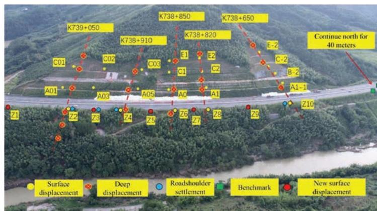
Figure 5 Layout of on-site monitoring points for slope.
