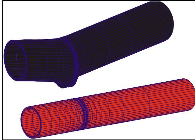
**Figure 15.** *Displaced structure during welding*
