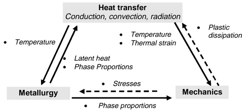
**Figure 1.** Interactions of physical phenomena in the solid during welding
