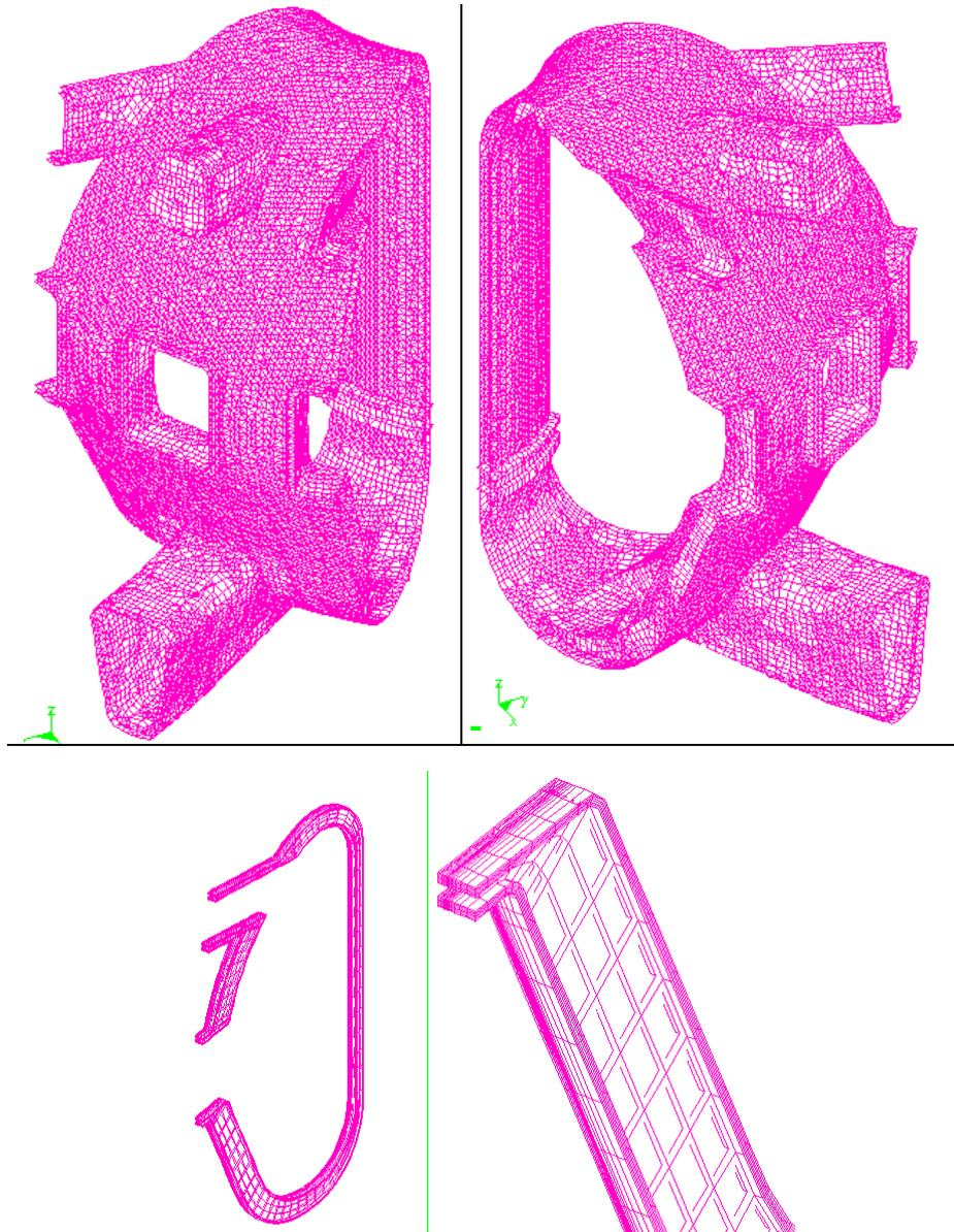
**Figure 20.** Global model and 3D elements (in and near welds)
