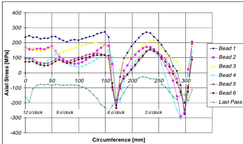
**Figure 16.** *Weld residual stresses in axial direction along the circumference of the weld*
