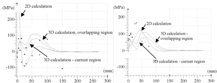
**Figure 11.** Hoop (left) and axial (right) stresses on the external pipe surface (from Duranton *et al.* 2004)
