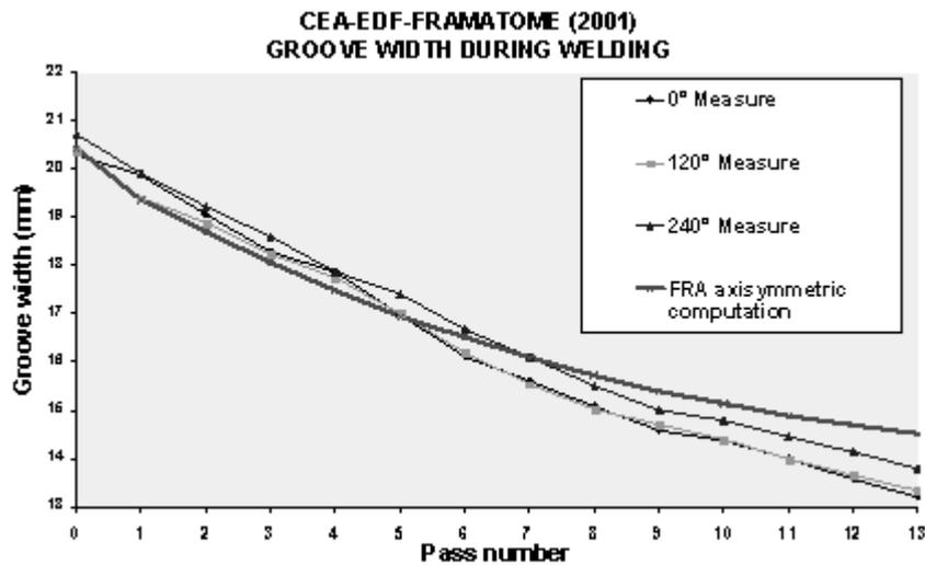
**Figure 8.** Measured and computed groove shrink during welding
