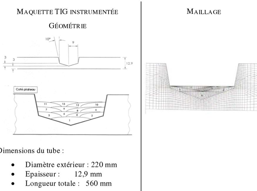
**Figure 7.** Scheme and mesh of the welding beads in the A13pipe mock-up
