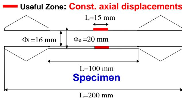
**Figure 3.** Scheme of the Satoh specimen, homogeneously heated under zero strain
