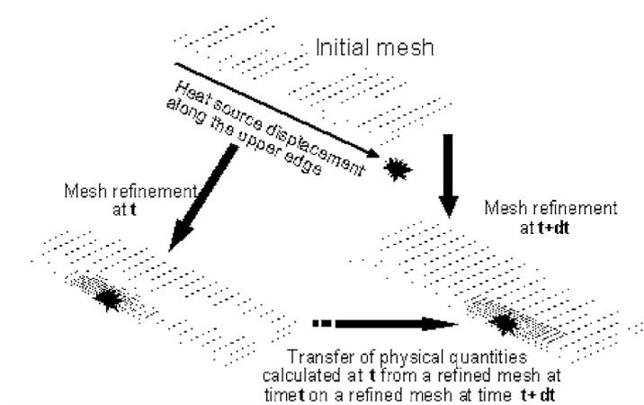
**Figure 10.** Moving mesh refinement (from Duranton *et al.*, 2004)
