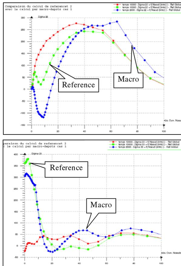
**Figure 9.** Validation of the macrobead technique: comparison of stresses on the outer pipe wall
