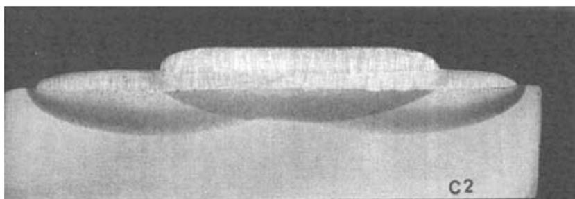
**Figure 21.** Macrography of the austenitic layer deposits on a Reactor Pressure Vessel (RPV) ferritic steel
