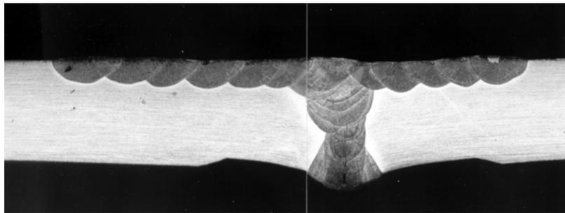
**Figure 13.** Cross section of the manual TIG weld including the LPHSW
