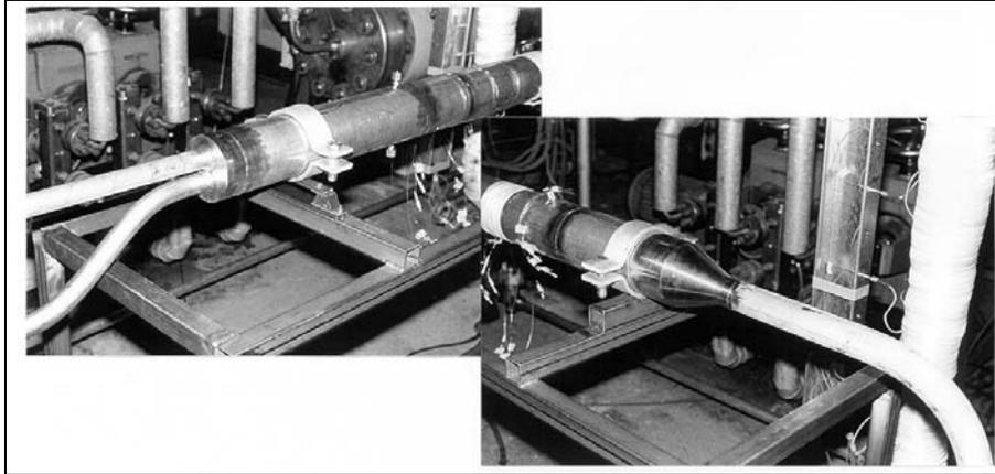
**Figure 12.** Test pipe assembled for aging tests
