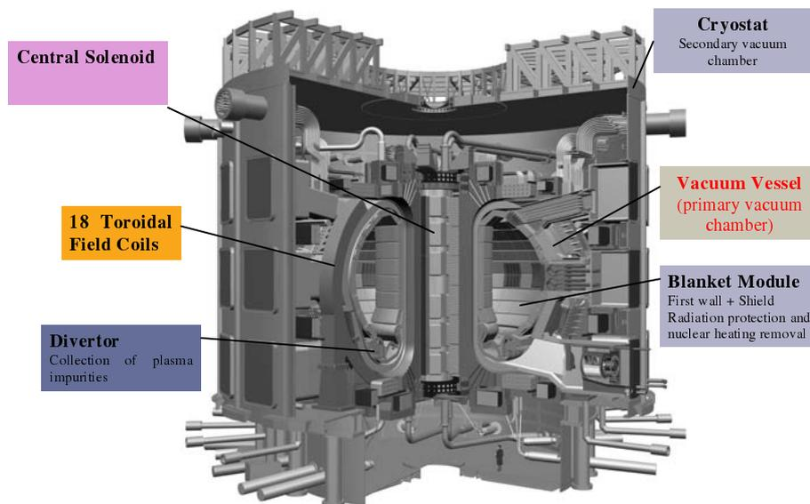
**Figure 17.** Exploded view of the ITER torus
