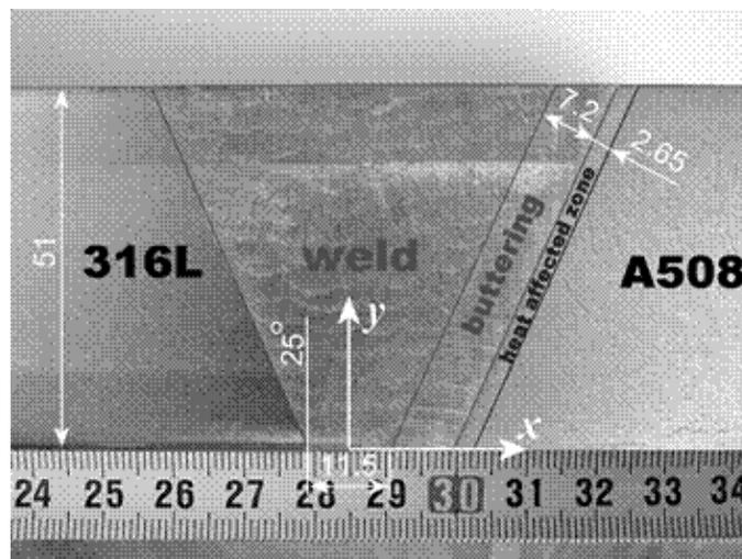
**Figure 22.** Cross-section of the bi-metallic weld of AD01 mock-up
