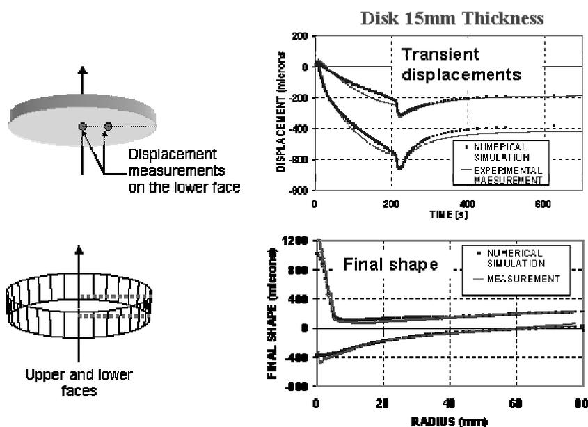
**Figure 6.** Comparison of measured and computed shapes of 316L disk
