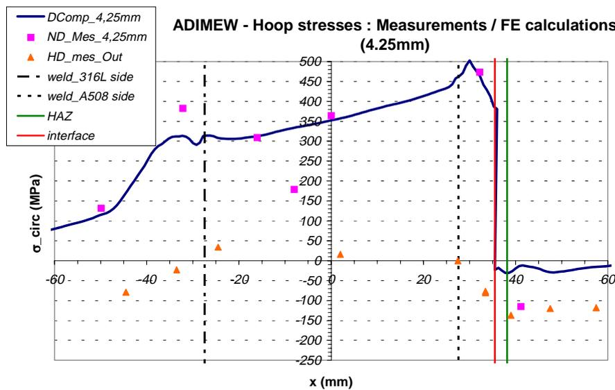
**Figure 23.** Hoop residual stresses at 4,25 mm under the outer wall
