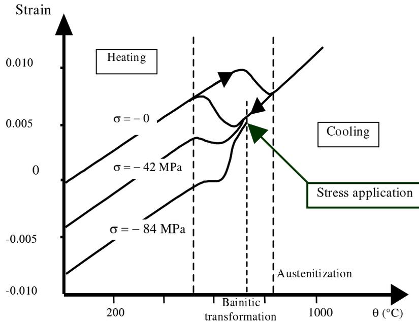
**Figure 2.** Combined dilatometry test
