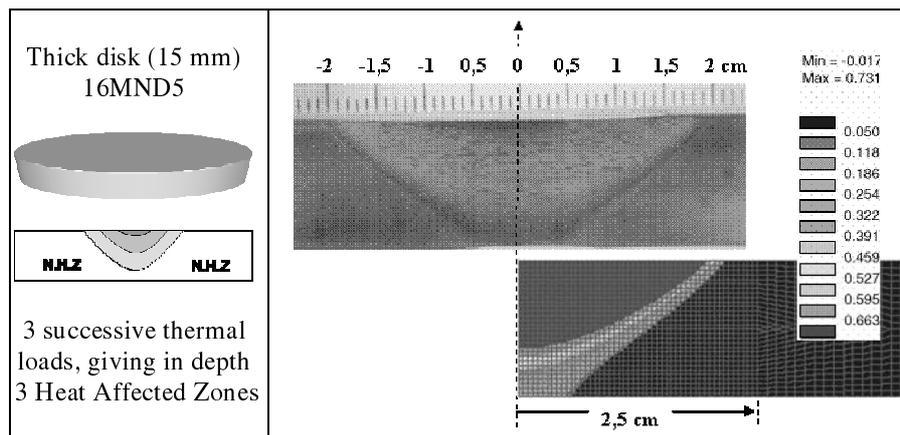
**Figure 5.** Comparison of measured and computed Heat Affected Zones in a disk
