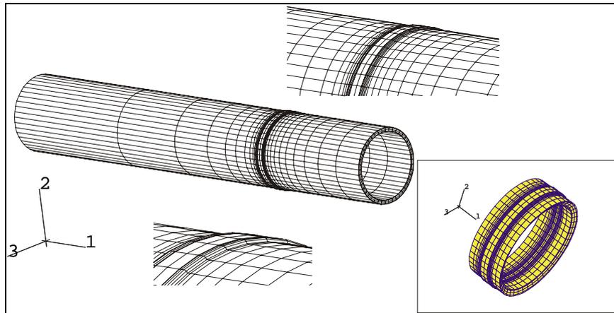
**Figure 14.** *Finite element mesh with details of the weld*
