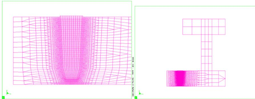
**Figure 19.** Local models for thermal and thermo-mechanical calculations (inner shell)
