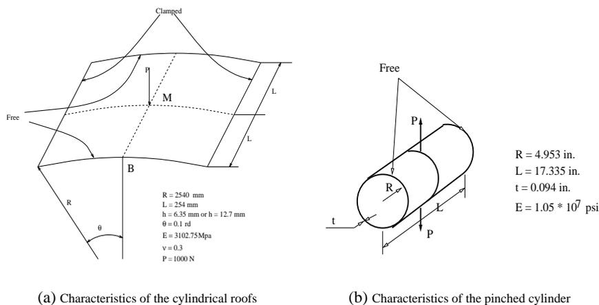
**Figure 1.** Description of the geometrically non-linear shell problems
