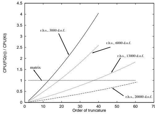
(b) Numerical cost of a series. Case of a non-symmetric tangent matrix. Navier-Stokes equations are discretized as in [CAD 01a]
