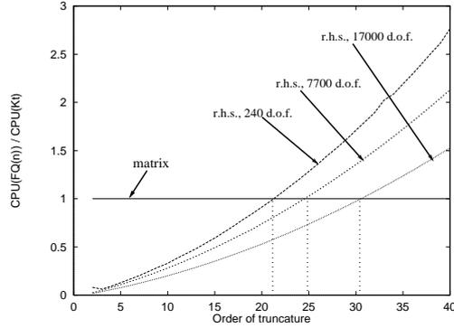
(a) Numerical cost of a series. Case of a symmetric tangent stiffness matrix. Shell problems of figure 2
