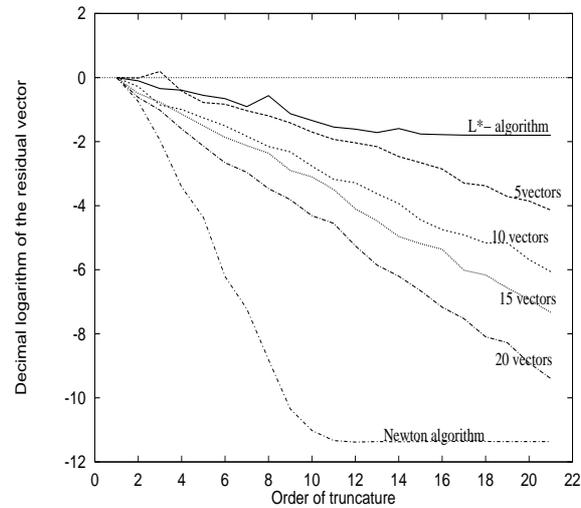
**Figure 7.** Iterative process defined in figure 6. Logarithm of the residual vector versus the order of truncature for the three high order correctors
