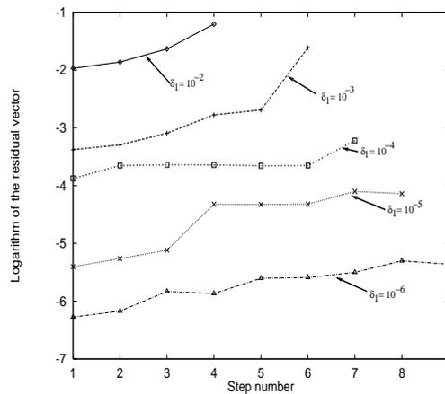
**Figure 5.** Thin cylindrical roof, DKT18 element. Evolution of the logarithm of the residual vector versus the step number and for various values of parameter  $\delta_1$ . Order of truncature 15
