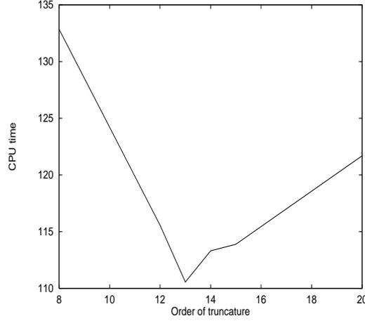
**Figure 3.** A typical curve CPU time versus truncature order, from [ABI 02]. It concerns a hemispherical deep drawing process, with 5766 dof. Here the optimal order is 13
