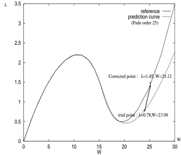
**Figure 6.** Response curve of the thick cylindrical roof. The trial and corrected points. Residual vector at the trial point is :  $\log_{10}(R^p) = 0.78$
