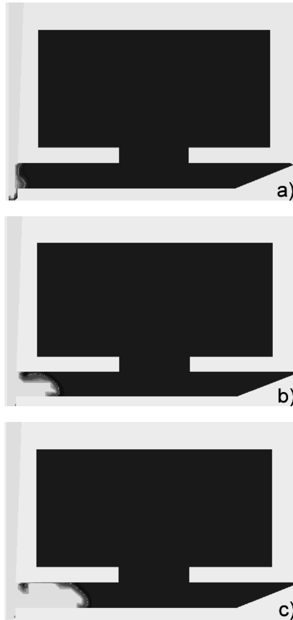
Figure 10. Numerical results achieved using the stabilized FE/FV method. The melt leaves the sprue (a) and enters the runner (b). Still the transition region remains compact (c)
