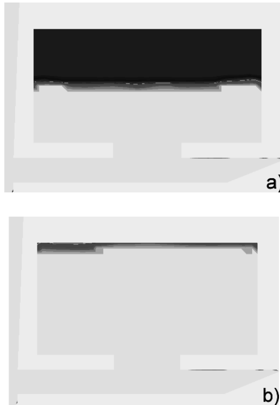
Figure 12. The plate is filled vertically (a). An almost plane front is observed. Using the stabilized FE/FV method the plate is filled at 2.65 seconds (b)
