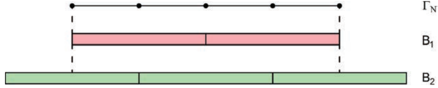
Figure 1 Schematic to show the block structure, where \Gamma_N is the surface over which the Neumann BC is being scaled, and B1 and B2 are the blocks over which the flux is redistributed.
