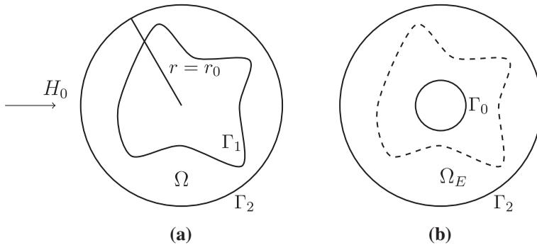
**Figure 1.** Cross-section of the annular-like pipe. Note: (a) original domain  $\Omega$  between  $\Gamma_1$  and  $\Gamma_2$ , (b) extended domain  $\Omega_E$  between  $\Gamma_0$  and  $\Gamma_2$ .
