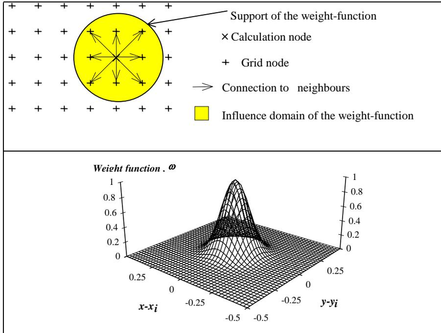
**Figure 1.** *Neighboring nodes and gaussian weight function*
