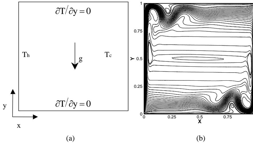
**Figure 3.** (a) Differentially heated square cavity (b) Streamlines for  $Ra=10^8$
