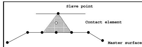
**Figure 2.** A representation of contact elements
