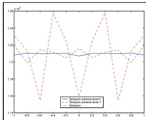
Figure 9. Normal contact multiplier  $\lambda$  on contact interface
