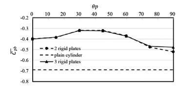
**Figure 11.** The mean base pressure coefficient,  $\overline{C_{pb}}$ , against attachment angle,  $\theta_{p'}$  in tri-splitters case compared with the plain cylinder and cylinder with two splitter plates.
