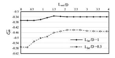
**Figure 14.** The mean base pressure coefficient,  $(\overline{C_{p_b}})$ , against the dimensionless length of the middle plate  $(L_{mid}/D)$  in two different cases:  $L_{lat}/D = .3$  and  $L_{lat}/D = 1$ .
