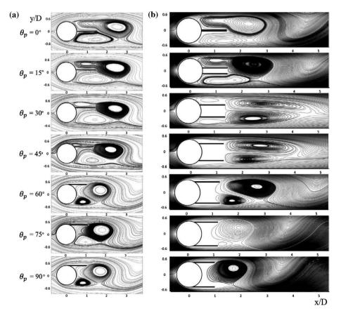
Figure 5. Instantaneous streamlines (a) cylinder with single-splitter and (b) cylinder with dual-splitters.
