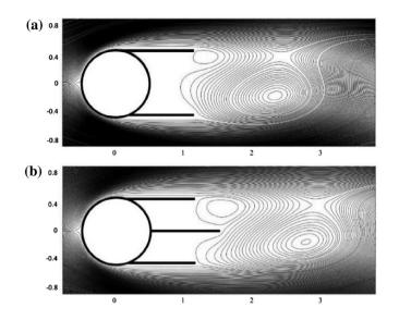
**Figure 6.** Instantaneous streamlines before lower vortex sheds at  $\theta_p = 75^\circ$  (a) cylinder with dual-splitters and (b) cylinder with tri- splitters.
