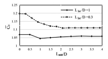
**Figure 12.** Mean drag coefficient,  $\overline{C_p}$ , against the dimensionless length of the middle plate ( $L_{mid}/D$ ) in two different cases:  $L_{lat}/D = .3$  and  $L_{lat}/D = 1$ .
