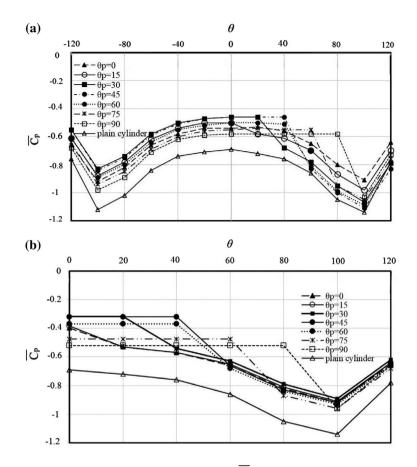
**Figure 10.** The mean pressure coefficient distribution,  $\overline{C_p}$ , against the angular position around the cylinder,  $\theta$ , in various attachment angle ( $\theta_p$ ) of splitter plates at downstream for (a) cylinder with single-splitter and (b) cylinder with dual-splitters.
