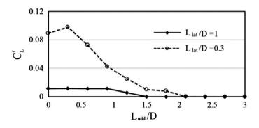
**Figure 13.** r.m.s. value of the lift coefficient ( $C'_L$ ), against the dimensionless length of the middle plate ( $L_{mid}/D$ ) in two different cases:  $L_{lat}/D = .3$  and  $L_{lat}/D = 1$ .
