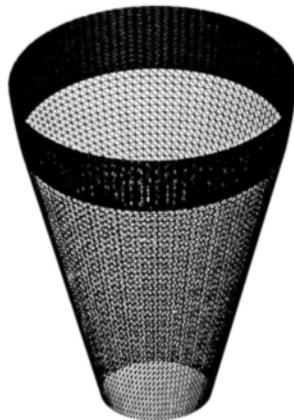
**Figure 1.** Finite element model of the nozzle
