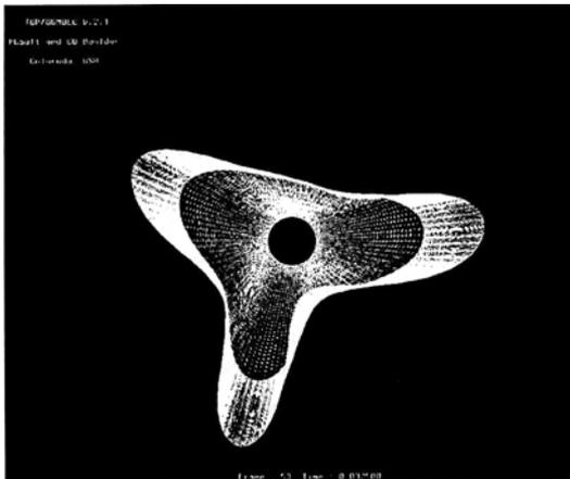
**Figure 18.** Behavior with a weaker stiffener and normal shock : shell shape just after a complete period : (artificial amplification by a factor 16)
