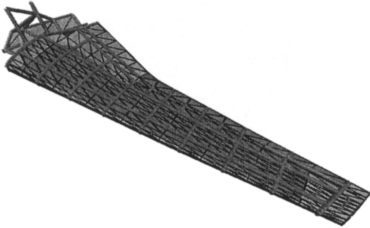
Figure 3. Reduced-Scale Model of a Wing Structure
