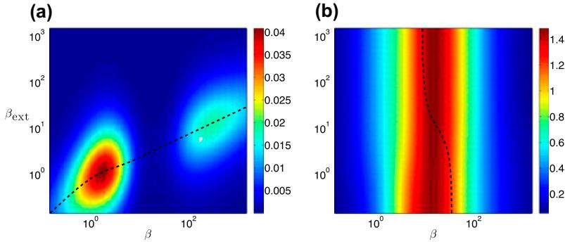
**Figure 4.** Non-dimensional harvested power  $\mathcal{P}$  (a) and internal dissipation  $\mathcal{P}_i$  (b) as a function of varying internal and external resistances  $\beta$  and  $\beta_{\text{ext}}$ . For both panels, the dimensional powers are scaled by  $\rho U_\infty^3 HL$ , and  $M^* = 1$ ,  $\alpha = 0.3$ ,  $H^* = 0.5$  and  $U^* = 15$ .
