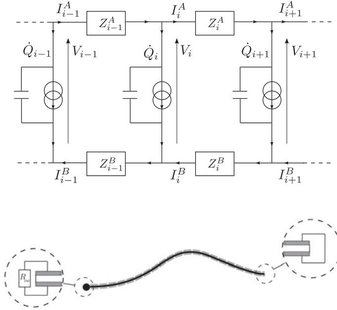
**Figure 2.** (Top) Local electric circuit: each piezoelectric pair is equivalent from an electric point of view to a current generator and an internal capacitance. The current through a patch pair and the voltage at its free electrodes are, respectively,  $V_i$  and  $\dot{Q}_i$ . (Bottom) Boundary conditions for leading edge harvesting, Equation (12).
