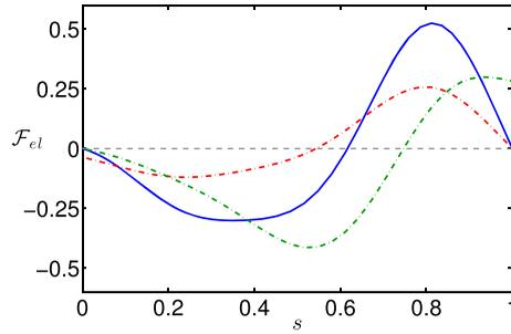
**Figure 5.** Comparison of the electrical energy fluxes  $\mathcal{F}_{el}$  with no harvesting resistor (blue) and for harvesting resistance at the leading or trailing ends (red and green, respectively)  $\alpha = 0.3$ ,  $H^* = 0.5$ ,  $M^* = 1$ ,  $U^* = 15$ ,  $\beta = 1.95$ ,  $\beta_{ext} = 1.05$  (optimal configuration on Figure 3).
