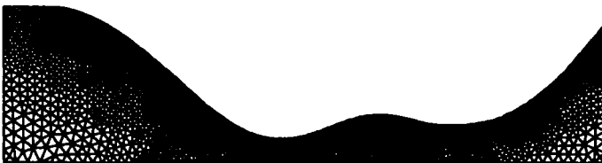
Figure 9.13. Ecoulement laminaire, maillage.
